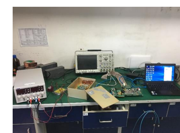
Test environment and result with TIGER ASIC (Radiation source: Cs 137 , with energy resolution of about 5%)
