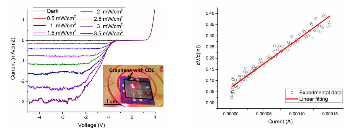
The results were compared with models and previous work, showing consistent results with a R<sub>s</sub>= 2 k $\Omega$ , an ideality factor of 2.66 and a  $\Phi_B$  of 1.01 eV.
