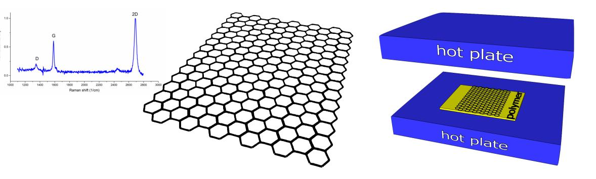
In order to avoid these problems, the idea of this work is to use a hot embossing machine to imprint the graphene from the Cu foil directly on a polymer substrate, avoiding the transfer steps and thus allowing better preserving the quality of the Graphene as it was just after the growth.
