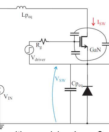
Such circuit includes the GaN model, an ideal diode and two global parasitics, an inductance and a capacitance, evaluated exploiting the procedure used for the snubber design. The load is a constant current source, while the driver is an ideal one.
