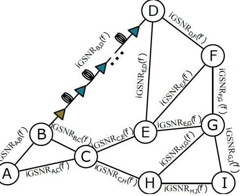
transmission line connecting two ROADM nodes including pre-amp and booster amplifiers. Each edge is characterized by a value of GSNR degradation (iGSNR(f,i)<sub>1 m</sub>) representing the QoT degradation introduced by each transmission line between node \$I\$ and node *m* for the
