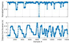
Strong non-linear dependence between sensor output and the distance to person Noise limited correlation between sensor data and distance of person from the sensor
