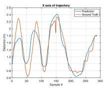
The resulting RMSE was about 26 cm, which is perfectly suitable to track, for example, the movement of an elderly person within an apartment
