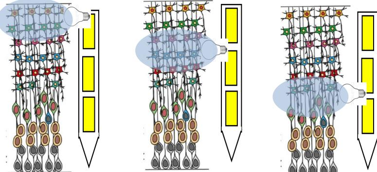
Voltage measure of neural extracellular action potential. Measure due to double layer capacitance formation at electrode interface
