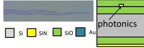
**3.Circuit integration on tip** combination of dry top wafer etch + wet bottom wafer etch **2.** Patterning of electronic circuits Electronics alignment to photonics, patterning (electron beam lithography + liftoff) electronics
