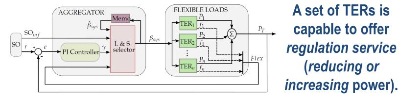
• Aggregator decides the set-point of each TER, based on a three-state signal (0,1, or-1).
