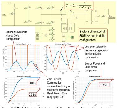
Phase Shift Control Implemented starting with DutyCycle = 0 to avoid current overshoot during the start-up.
