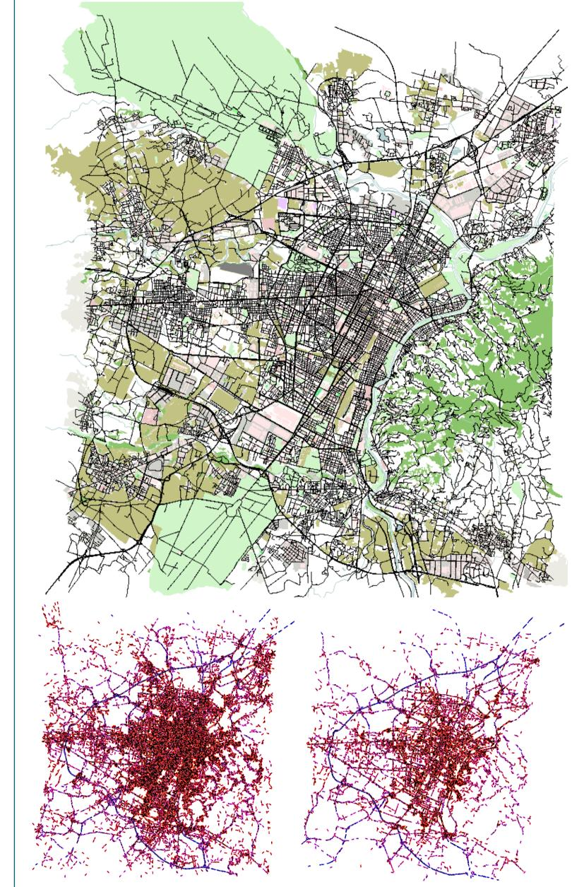
• OSM data were converted in a network file of SUMO-readable XML format, to create the map of the model. Unfortunately the procedure described leads to a network with many errors, so some **manual correction** were needed (average velocities, number of lanes, roundabout connectivity, traffic lights phases and synchronization).
