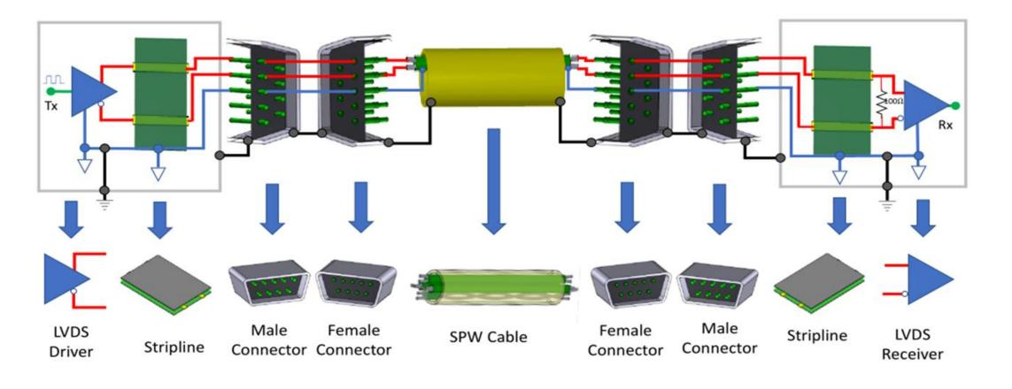
Development of **full-wave 3D models** for short components and **2D models** for transmission lines, with all blocks combined in SPICE simulations
