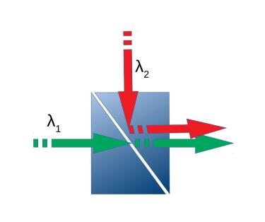
• Development of **multiplexing technologies for power** scaling. Typical module power scaling is obtained by combining spatial and polarization multiplexing. However these approaches are quickly reaching their limit, particularly for higher beam quality applications.
