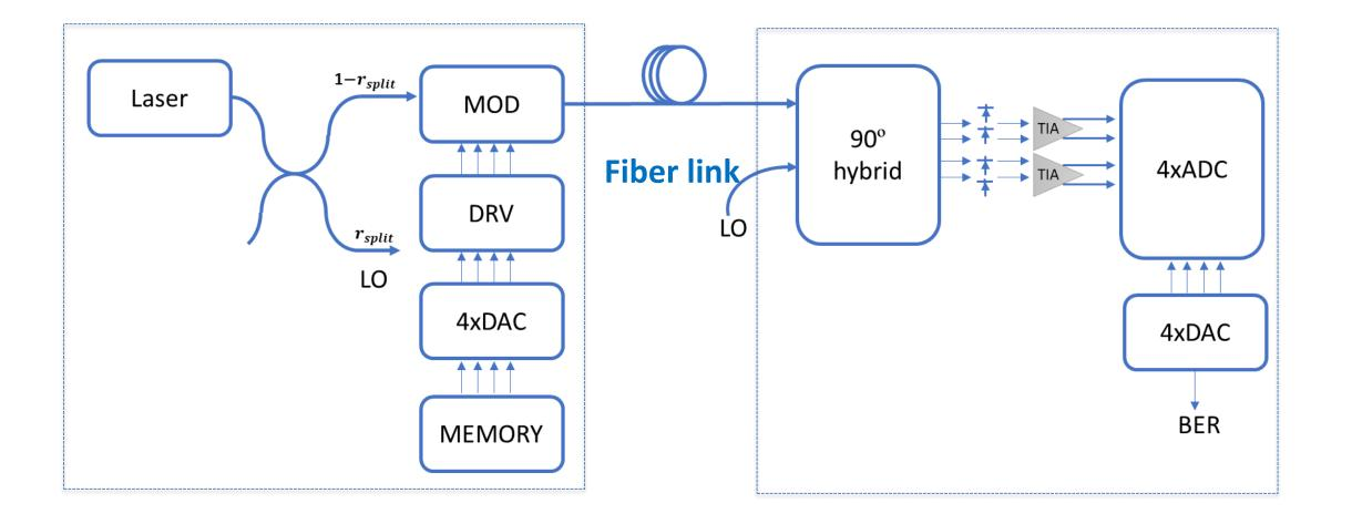
• The architecture at the transmission part is similar as the used in long haul coherent
