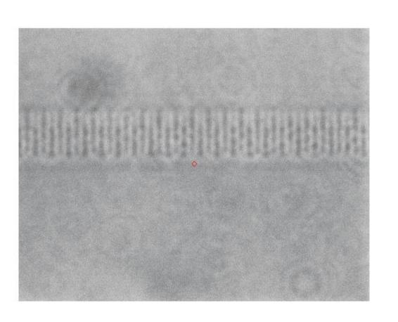
Direct-written short-wavelength Fiber Bragg Gratings (FBGs) in silicate and softglass fibers using a femtosecond laser. These gratings are more challenging than those used in optical communications or for sensing because of the much shorter wavelength. A special recipe using the "Line-by-Line" technique and high Bragg orders (4-10) has been developed for fibers, starting from silicate Output the (OC)Coupler because its lower OŤ reflectivity.
