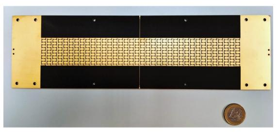
**Principle of operation:** the lower metasurface acts as an electronically-controlled, variable-impedance plane; changing the value of such impedance affects the phase velocity of the traveling wave and, therefore, the radiation angle.
