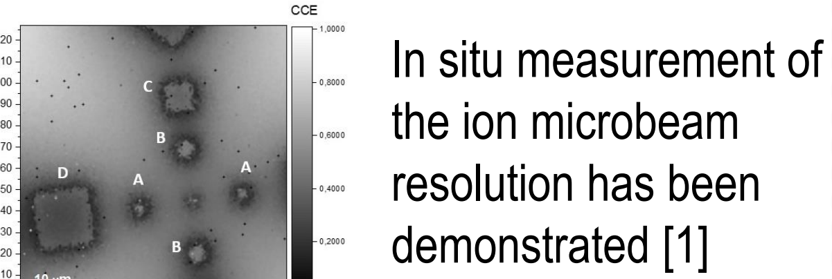
IBIC map of a FIB machined Si photodiode
