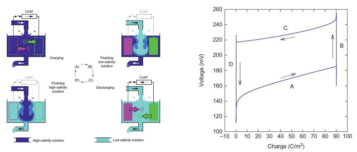
Area of charge-voltage plot is proportional to the harvested energy. In charged state, the change of the electrolyte (in OCV conditions) produces a voltage rise in order to satisfy **Q=CV**
