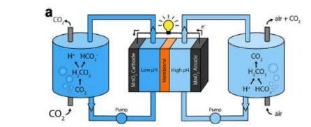
Different amount of CO<sub>2</sub> in 2 different tanks of water produces a pH difference. Exploiting a semipermeable membrane, it is possible to generate a pH gradient, resulting in a voltage drop across the device.
