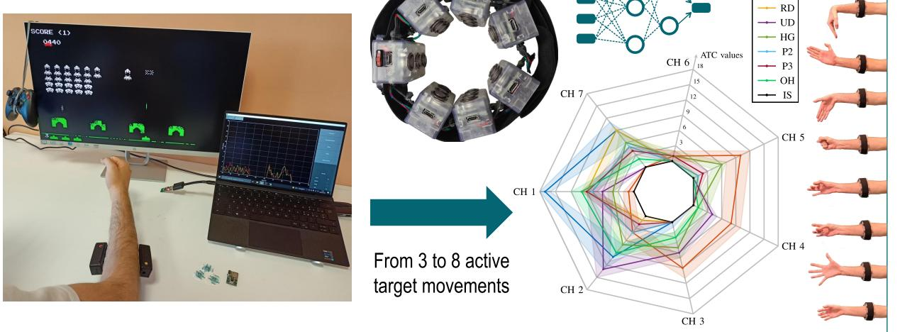
By combining our acquisition boards, we designed an armband consisting of 7 channels and able to distinguish among 8 gestures, plus an idle state, with an accuracy of 91.9%. Using ATC as the only feature for classification allowed us to achieve a total current absorption of **2.92 mA**, with latency due to prediction of only **1.34 ms**.
