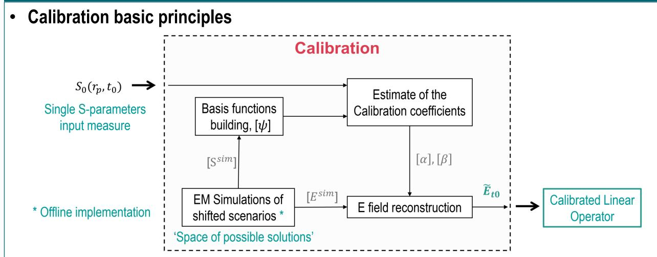
This technique can compensate for **several variables** of different natures, from physical inaccuracies in the probes to the external electronics phase shifts. Moreover, it can be
