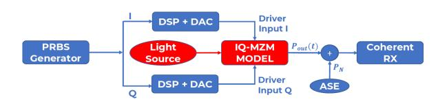
For back-to-back time-domain simulations the Python model has been inserted in a more complex split-step Fourier method (SSFM) modulator.
