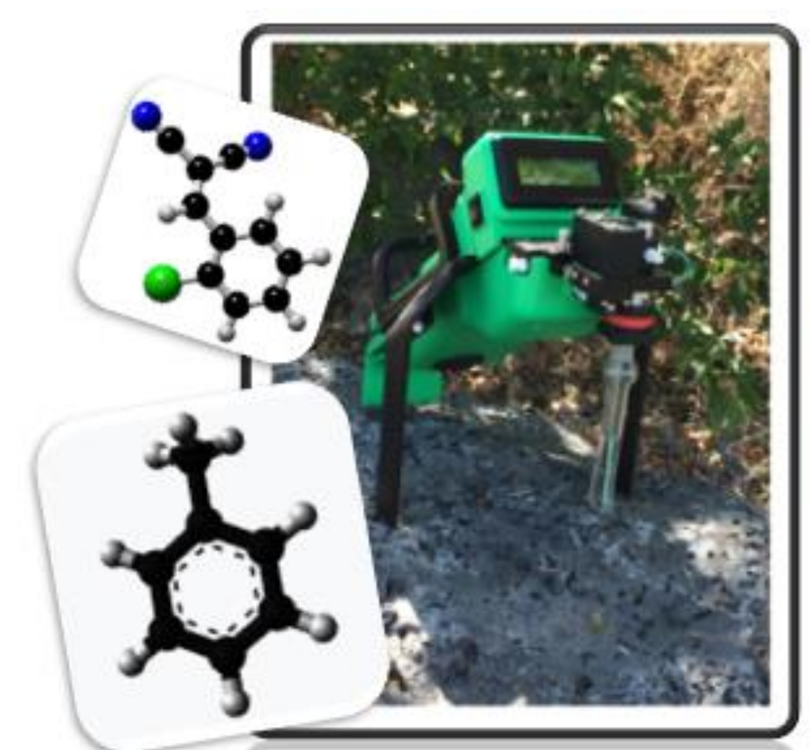
Figure 5: Example of portable GC for hydrocarbon detection
